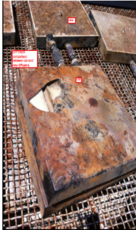
Defective diffusers that were replaced almost a week earlier
