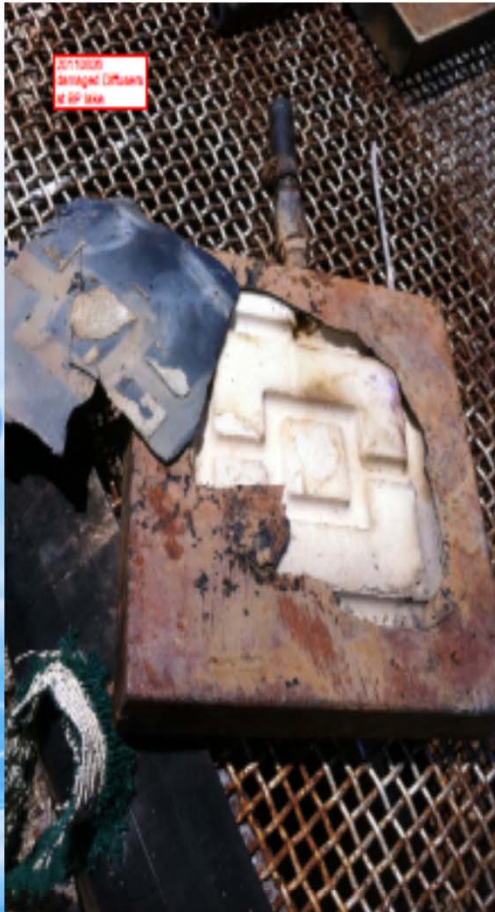
Defective diffusers that were replaced almost a week earlier
