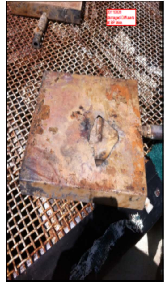
Defective diffusers that were replaced almost a week earlier
